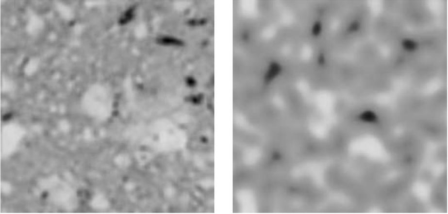
**Fig. 6.** 2D density image of a Loess soil (left, natural height 110 mm, resolution 0.44 mm) and a Gaussian random field (right) with equivalent grey level distribution and correlation length.
