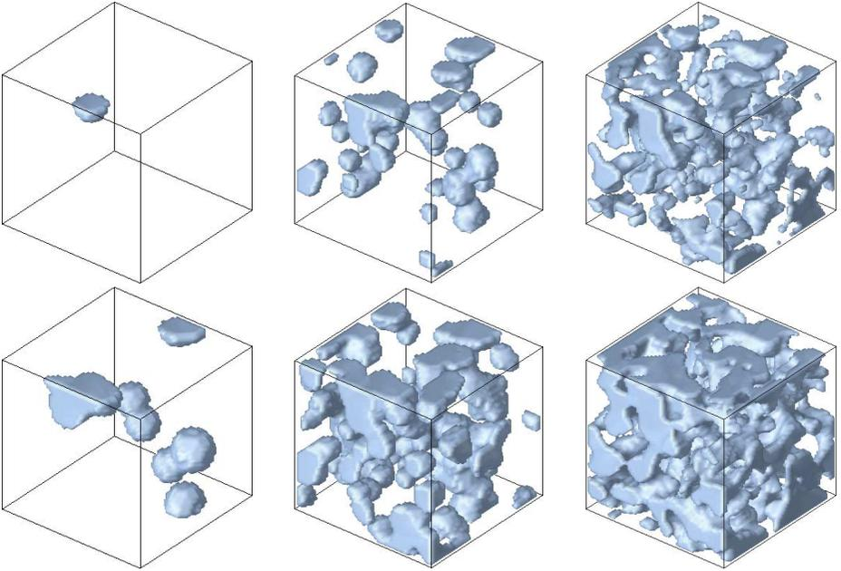
**Fig. 2.** Simulated pore structures from excursion sets according to different thresholds  $t = 100$  upper row and  $t = 120$  lower row. From left to right: isosurfaces for pores  $\mathbb{P}_{\text{op}}(d)$  with decreasing minimum diameter  $d$ . The related connectivity functions are shown in Fig. 3.
