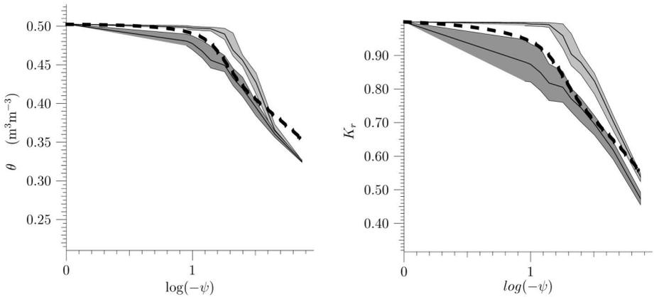
**Fig. 5.** Water characteristic  $\theta(\psi)$  (left) and hydraulic conductivity function  $K(\psi)$  (right) obtained from network models with random topology (light grey) and measured topology of a Loess soil (dark grey). The shaded areas enclose the maximum and minimum values of 20 realizations. The dashed line represents the experimental results obtained for the Loess soil. The capillary pressure  $\psi$  is in hPa.
