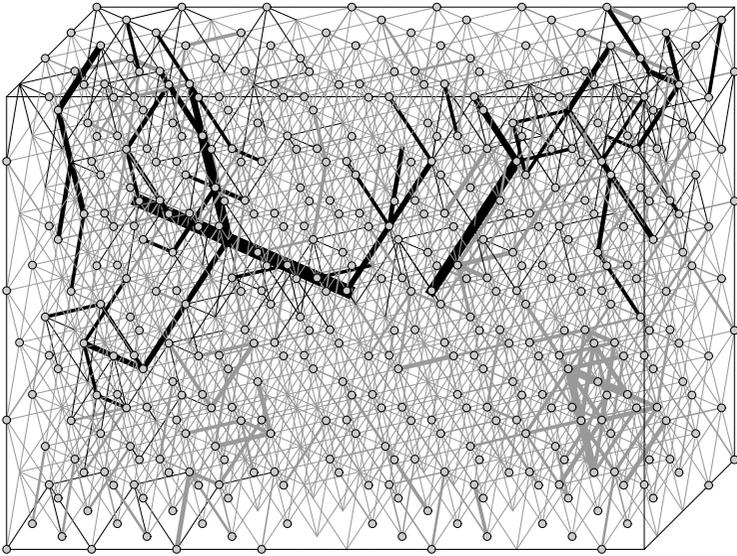
**Fig. 4.** Example of a networkmodel of  $8^3$  nodes at a certain capillary pressure where some pores are filled with water (grey) and others with air (black).
