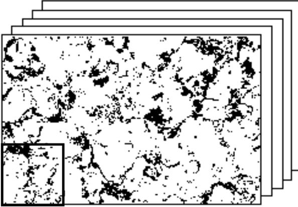
**Fig. 1.** One of 20 serial sections through undisturbed silty clay soil used to determine the Euler characteristic. Natural width is 20 mm, resolution is 0.013 mm/pixel, separation of serial sections is 0.4 mm, pores are black. The square in the lower left corner represents the size of a cube having the same volume as a pair of serial sections.
