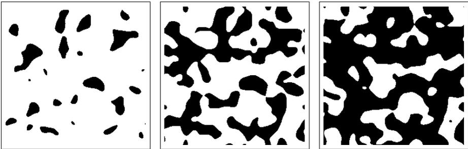
**Fig. 9.** Gaussian random field of Fig. 6 binarized according to different thresholds  $t = 140, 150, 160$  (from left to right)
