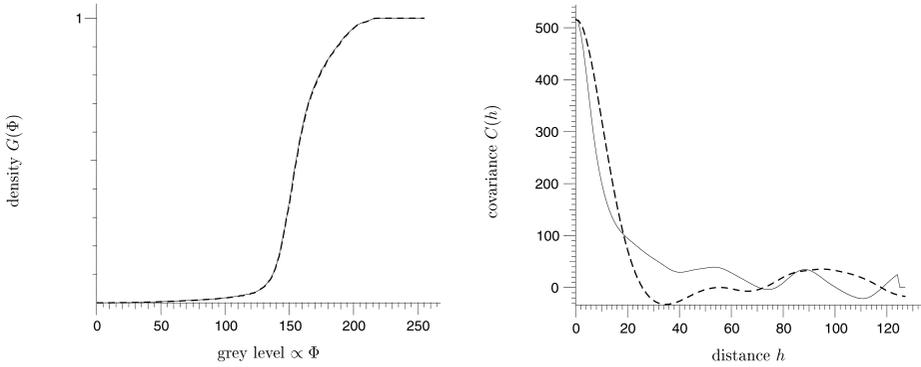
**Fig. 7.** Density function of porosity  $G(\Phi)$  (left) and auto-covariance  $C_{\Phi}(h)$  (right) for the natural structure of soil (thin line) and the correlated random field (dashed line) shown in Fig. 6.
