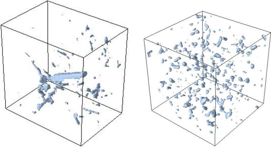
**Fig. 10.** 3D porosity image of a Loess soil (left, natural height 110 mm, resolution 0.44 mm) and Gaussian random field (right) with equivalent grey level distribution and correlation length. Grey levels below 40 indicating high porosities are marked by isosurfaces.
