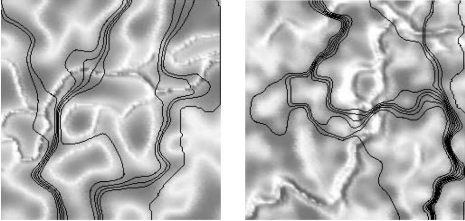
**Fig. 14.** Field of permeabilities (grey level) and velocity (elevation) together with iso pressure lines for stationary convective flow through the random fields  $f_1$  (left) and  $f_2$  (right). The effective permeability  $K_{\text{eff}}$  of  $f_1$  is by a factor of 71.5 larger compared to  $K_{\text{eff}}$  of  $f_2$ .
