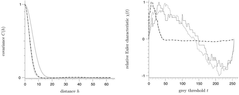
**Fig. 13.** Covariance and connectivity function for the random fields  $f_0$  (line),  $f_1$  (dashed line), and  $f_2$  (dotted line). The connectivity functions are normalized by the maximum value of  $\chi(t)$  for better comparison.
