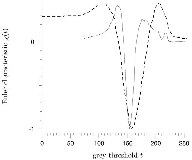
**Fig. 11.** 3D connectivity function  $\chi(t)$  for the 3D X-ray image of soil (line) and the Gaussian random field (dashed line). The Euler characteristics are plotted relative to the maximum value to allow a better comparison of the two curves. The images are shown in Fig. 10
